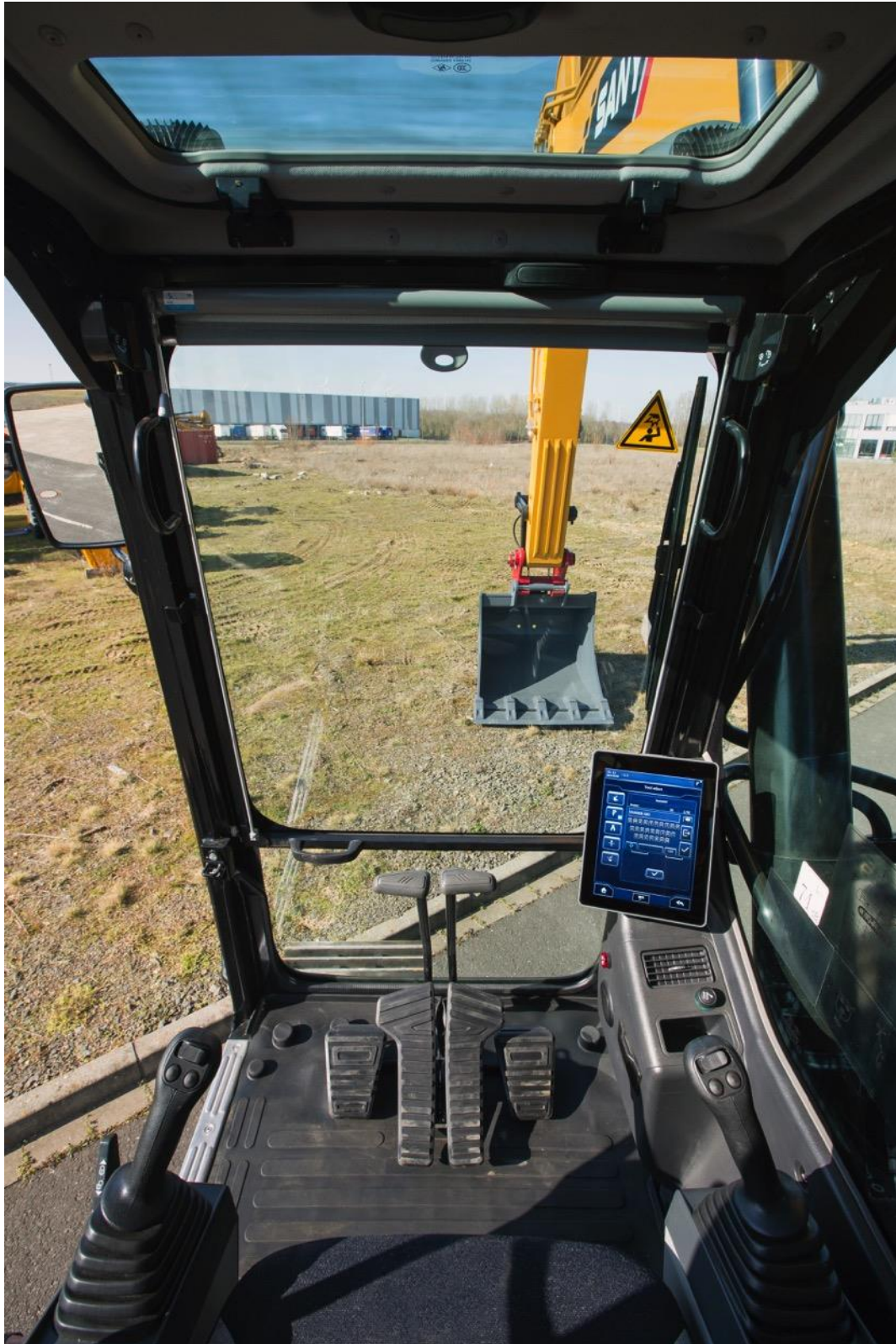
Image 2: Comfortable cab with high-resolution 10" touchscreen display for images and simple operation
