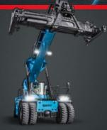
REACH STACKER SRSC45E5 Battery capacity 422 kWh Load capacities at row 1 / 2 / 3 45 / 31 / 15 t Wheel base 6000 mm Axle Kessler
