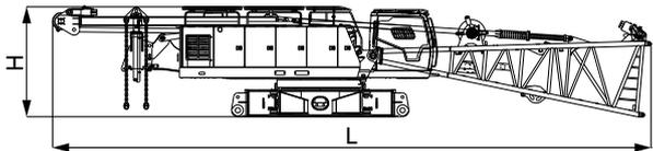
**Basic Machine (Mode 2: with A-frame, rear counterweight self-assembly device, boom base, reeving winch and jib luffing winch)** ×1
