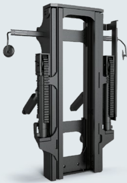
Optional - duplex mast with free lift: Lift cylinder on duplex mast with free lift positioned to the side of the mast, thus unrestricted view through the central free space of the mast
